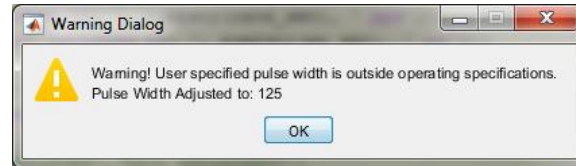
Figure 5. Warning dialog display when the pulse width specified has been adjusted to meet operating specifications.
