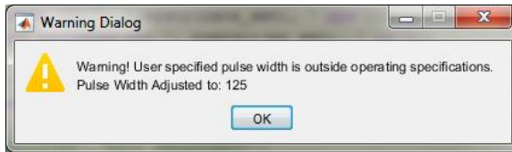
Figure 3 (left). Warning dialog display when the pulse width specified has been adjusted to meet operating specifications. Figure 4 (right). Warning dialog display when the stimulation rate has been decremented to meet the total stimulation rate allowed.
